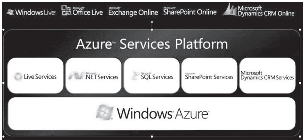
**Figure 2.6** The Windows Azure architecture and framework. At the bottom level is the Windows Azure operating system. This runs in the virtualization environment created by Microsoft’s Hypervisor running on bare hardware. At the top layer are end-user applications, which Microsoft is recasting to be delivered as SaaS. Source: Microsoft.
